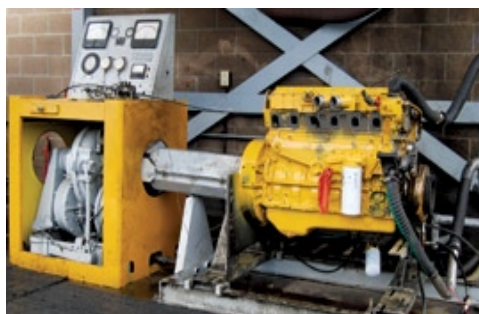
Engine Dynamometer Testing
